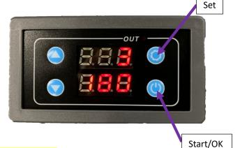
P1--2: Relay will ON after delay T1. Then Relay will OFF after delay
